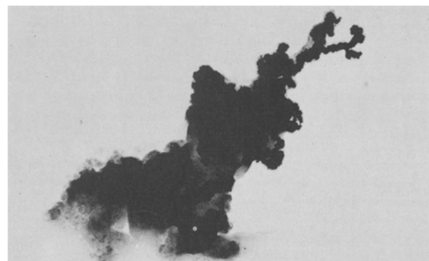
FIG. 5. A particle of platinum on activated carbon (x 62,500).
